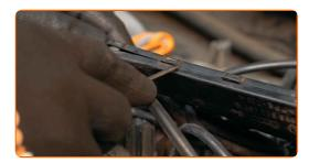
Make marks on the distributor cap to indicate the installation order of the spark plug wires.
