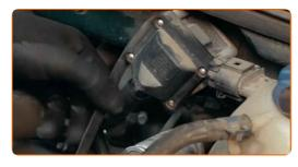
14 Attach the spark plug wire bracket.
