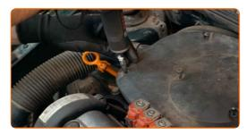
Remove the air filter housing.
