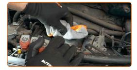
Install the air filter housing and fasten it. Use a Phillips screwdriver.
