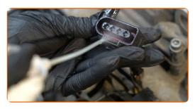
Plug in the connectors of the ignition coils.
