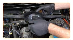
Pour coolant in the coolant reservoir.
