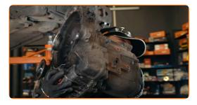
Remove the release bearing. Use a crowbar.
