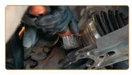
90 Install the steering knuckle on the CV axle.
