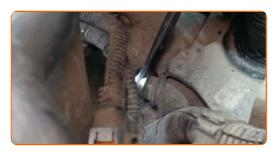
Remove the bottom gearbox mount.
