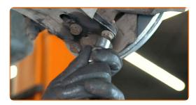
Attach the transmission sensor connector.
