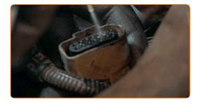
Connect the engine wiring harness connector.
