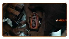
Detach the engine wiring harness.
