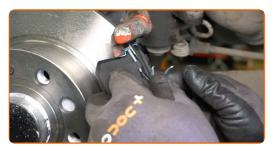
Install the brake caliper and fix it. Use a combination spanner #13. Use a combination spanner #15.
