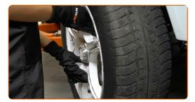
Remove the dust boot caps of the brake caliper guide pins. Use a crowbar.
