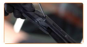
Remove the blade from the wiper arm.
