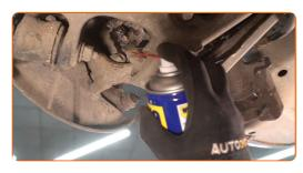
Unscrew the caliper bracket fastening. Use HEX No.H8.
