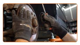
15 Remove the brake disc.
