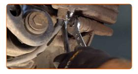
Remove the brake caliper. Use a crowbar.
