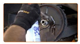
Install the new wheel hub with a bearing.
