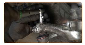
Tighten the fastening nut connecting the tie rod end to the steering knuckle. Use a drive socket #15. Use a torque wrench. Tighten it to 45 nm torque.
