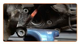
Unscrew the wheel hub axle nut. Use XZN #12. Use a ratchet wrench.
