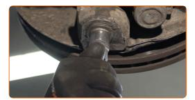
Tighten the ball joint fastener. Use a combination spanner #18. Use a torque wrench. Tighten it to 110 Nm torque.
