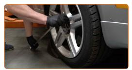
Loosen the fastener of the driveshaft. Use HEX No.H17. Use a tap wrench.
