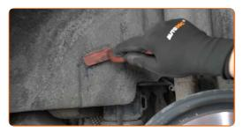
Unscrew and remove the wheel arch cover fasteners. Use Torx T25. Use a ratchet wrench.
