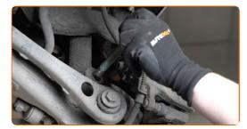
Clean the shock absorber fasteners. Use a wire brush. Use WD-40 spray.
