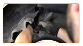
Remove the support from under the arm.
