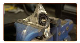
Tighten the shock absorber rod nut. Use a shock absorber socket DD№6. Use a drive socket #18. Use a torque wrench. Tighten it to 35 nm torque.
