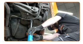
Tighten the lower fastener of the shock absorber. Use a combination spanner #21. Use a drive socket #21. Use a torque wrench. Tighten it to 150 Nm torque.+90°
