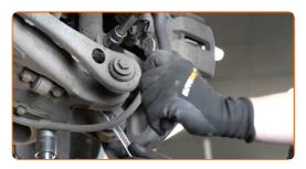
11 Remove the fastening bolt.
