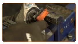
Remove the shock absorber piston rod fastening. Use a shock absorber socket DDNº6. Use a drive socket #16. Use a ratchet wrench.
