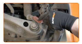
Unscrew the lower fastener of the shock absorber. Use a combination spanner #21. Use a drive socket #21. Use a tap wrench.
