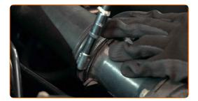
Unscrew the MAF sensor fasteners. Use a drive socket #10. Use a ratchet wrench.
