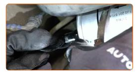
Screw in the fuel filter mounting bracket. Use a drive socket #7. Use a ratchet wrench.
