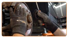
17 Remove the brake disc.
