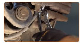
10 Remove the brake caliper. Use a crowbar.
