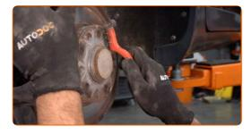
Remove the retaining ring. Use a crowbar.
