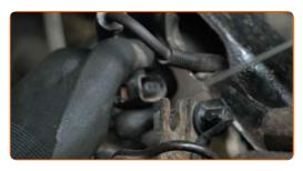
Disconnect the brake pads wear sensor. Use a crowbar.
