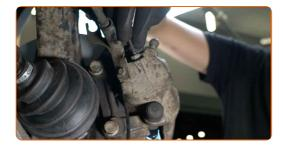
Connect the brake pads wear sensor.
