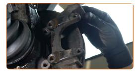
18 Remove the brake disc.
