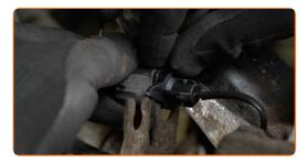
Connect the brake pad wear sensor plug.
