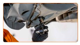
Tighten the fastener connecting the stabilizer bar with the control arm. Use a drive socket #13. Use a torque wrench. Tighten it to 25 Nm torque.
