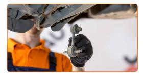
Replacement: anti roll bar links – SEAT Exeo ST (3R5). Tip:
