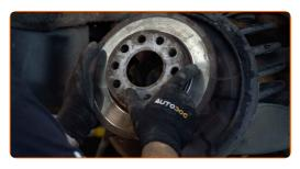
Remove the hub bearing protection cap. Use a hammer. Use a crowbar.
