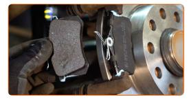
Install the brake caliper and fix it. Use a drive socket #13. Use a combination spanner #15. Use a torque wrench. Tighten it to 35 Nm torque.
