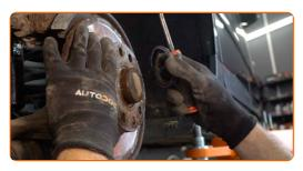
15 Remove the brake disc.
