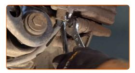
Remove the brake caliper. Use a crowbar.
