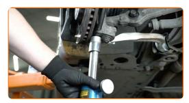
Tighten the rear fastener connecting the arm to the body subframe. Use a combination spanner #18. Use a drive socket #18. Use a torque wrench. Tighten it to 70 Nm torque.+180°
