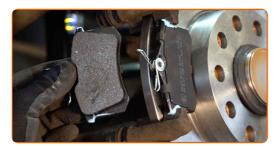
Install the brake caliper and fix it. Use a drive socket #13. Use a combination spanner #15. Use a torque wrench. Tighten it to 35 Nm torque.
