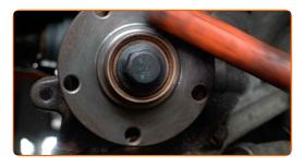
20 Install the brake disc.
