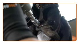
17 Remove the caliper bracket.
