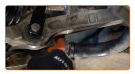
Install a new rod, tighten the fasteners. Use a combination spanner #16.
