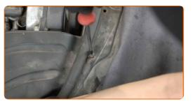
23 24 Remove the fender protection cover.
