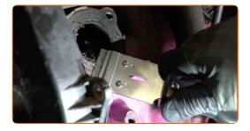
Treat the water pump mounting seat. Use a sealant.
