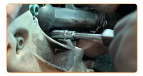
Remove the thermostat housing.
