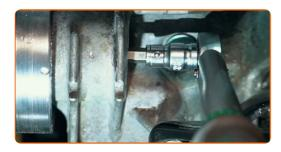
Pull aside the V-ribbed belt tensioner pulley. Use a combination spanner #17.
