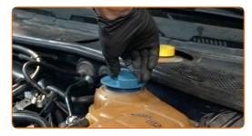
Screw on the coolant reservoir cap.
