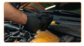
Pour coolant in the coolant reservoir.
