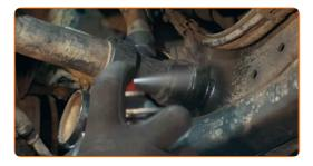
Disconnect the coolant pipe retaining clip.
