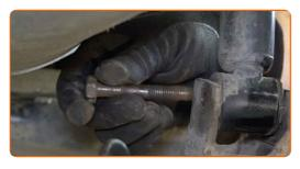
18 Remove the suspension strut.
