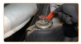
Loosen the upper fastener of the shock strut mount. Use a combination spanner #17. Use a shock absorber socket #DD5,2. Use a ratchet wrench.
