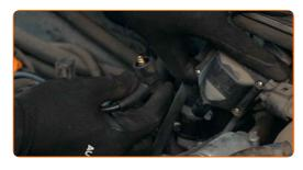
Connect new spark plug wires to the distributor cap.
