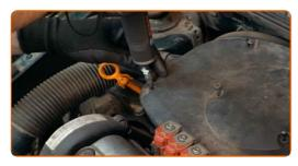
Remove the air filter housing.
