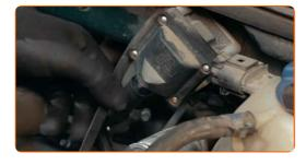
14 Attach the spark plug wire bracket.
