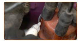
Disconnect the spark plug wires from the distributor cap.
