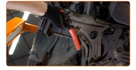
Unscrew the fastener connecting the stabilizer bar with the control arm. Use a drive socket #13. Use a ratchet wrench.
