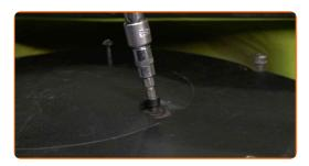
Tighten the fastening screws of the air filter cover. Use HEX No.H5. Use a torque wrench. Tighten it to 8 Nm torque.
