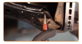
Tighten the fasteners of the ball joint. Use a drive socket #13. Use a torque wrench. Tighten it to 20 Nm torque.+90°
