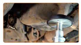
19 Install the front fastener of the arm.
