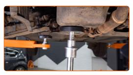
Remove the fastening bolt. Use a crowbar. Use a rubber mallet.
