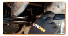
Screw the front arm fastener. Use a combination spanner #18.
