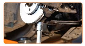
Tighten the front fastener connecting the control arm to the subframe. Use a drive socket #18. Use a torque wrench. Tighten it to 70 Nm torque.+90°
