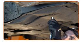
Remove the lower sound insulation.
