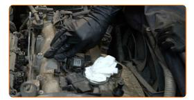
Tighten the chassis (ground) terminal of the ignition coils. Use a drive socket #10. Use a ratchet wrench.
