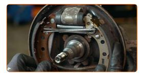
Install the retainers of the drum brake shoes. Use a brake shoe retaining spring compressor.
