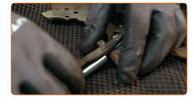
Install the upper retaining springs and adjustment mechanism on new brake shoes. Use a flat screwdriver.
