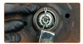
Unscrew the hub nut. Use a drive socket #24. Use a ratchet wrench.
