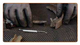
21 Install the brake shoe adjuster lever.
