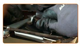
Install the brake shoes on the working brake cylinder on the bracket and on the brake-support plate bracket.
