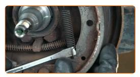
Disconnect the parking brake cable. Use a crowbar.
