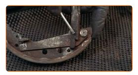
Remove the brake shoe adjuster lever.
