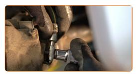
Unscrew the fastener connecting the brake hose to the brake circuit pipe. Use a combination spanner #11.
