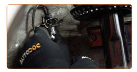
Tighten the fastener connecting the brake pipe to the brake caliper. Use a drive socket #11. Use a torque wrench. Tighten it to 30 Nm torque.
