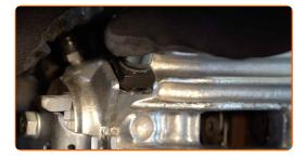
Tighten the fastener connecting the brake pipe to the brake caliper. Use a drive socket #13. Use a torque wrench. Tighten it to 35 Nm torque.
