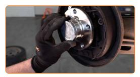
Treat the hub where it contacts the brake disk. Use copper grease.
