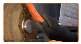
Treat the contacting surface. Use copper grease.
