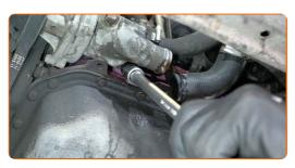
Remove the thermostat housing.
