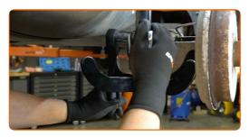
Unscrew the top fastening of the shock strut mount.
