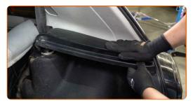
Screw the fasteners of the side plastic trim panel. Use a drive socket #10. Use a ratchet wrench.
