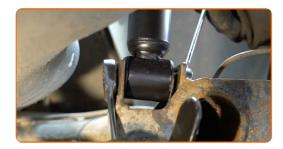
Tighten the lower fastening of the shock absorber. Use a combination spanner #17. Use a drive socket #17. Use a torque wrench. Tighten it to 70 nm torque.
