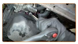
Remove the thermostat housing.
