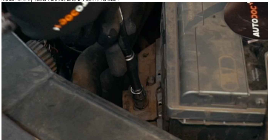
6 Remove the battery.
