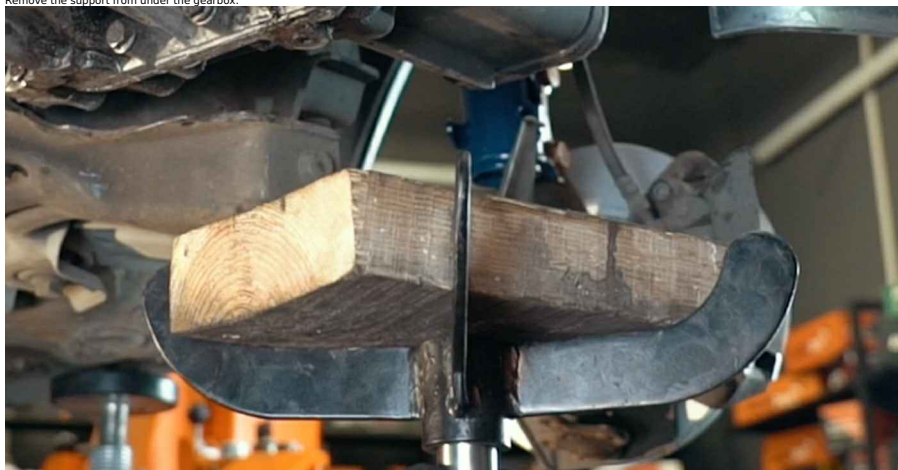
AUTODOC recommends: • Replacement: clutch kit - SEAT Cordoba Saloon (6K1, 6K2). Lower the transmission jack smoothly, without jerks, to avoid damaging components and mechanisms.
