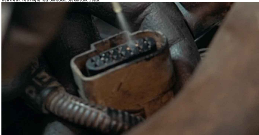
113 Connect the engine wiring harness connector.
