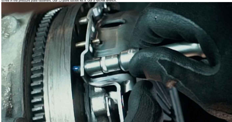
57 Align the clutch disc. Use a crowbar.
