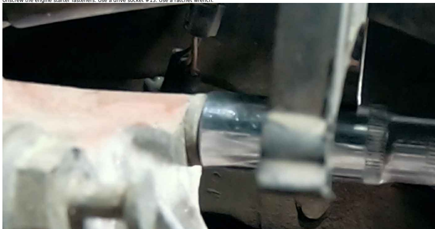
club.autodoc.co.uk 5-32 15 Unscrew the fasteners that connect the gearbox to the engine block. Use a drive socket #18. Use a ratchet wrench.
