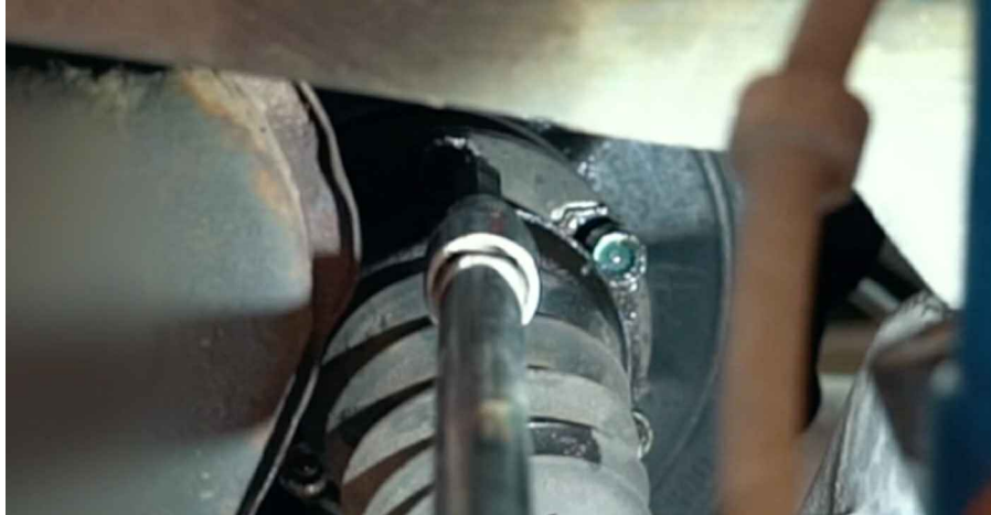
30 Remove the drive shaft.
