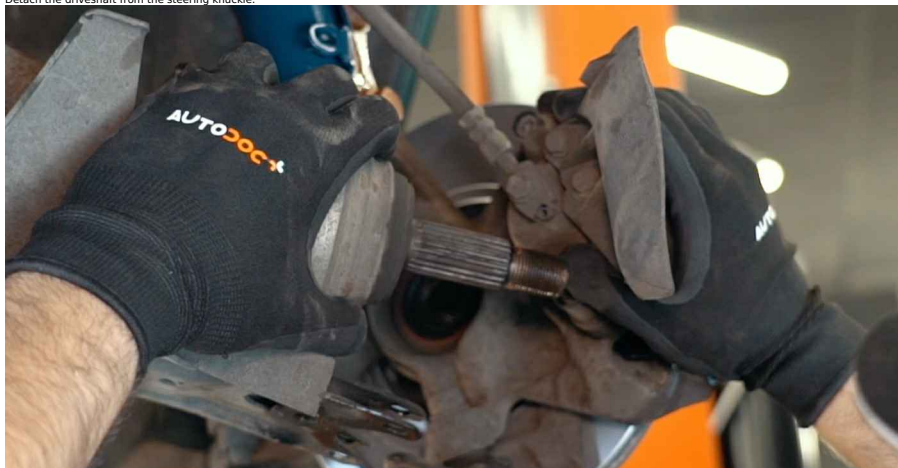
Replacement: clutch kit - SEAT Cordoba Saloon (6K1, 6K2). Tip: • Make sure that the drive shaft is not unloaded (when the car is jacked).
