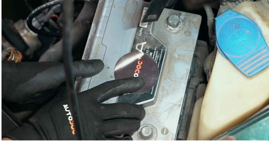
118 Screw in the battery fastener. Use a drive socket #13. Use a ratchet wrench.
