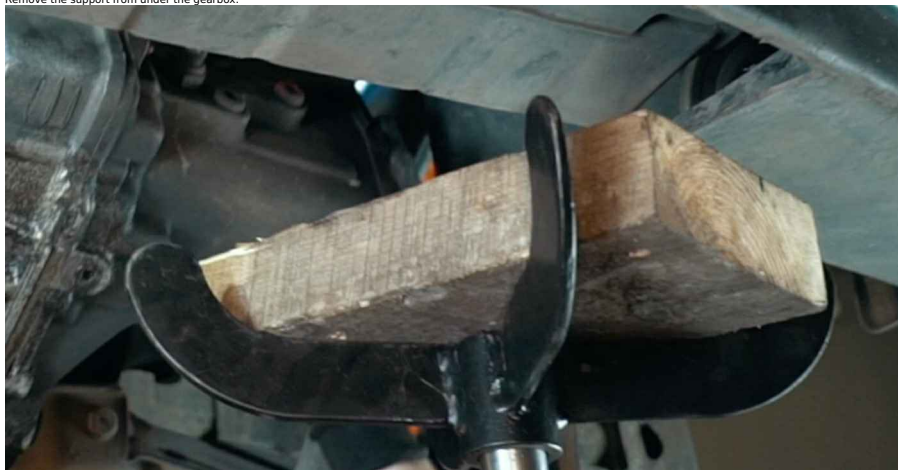
49 Remove the support from under the gearbox.
