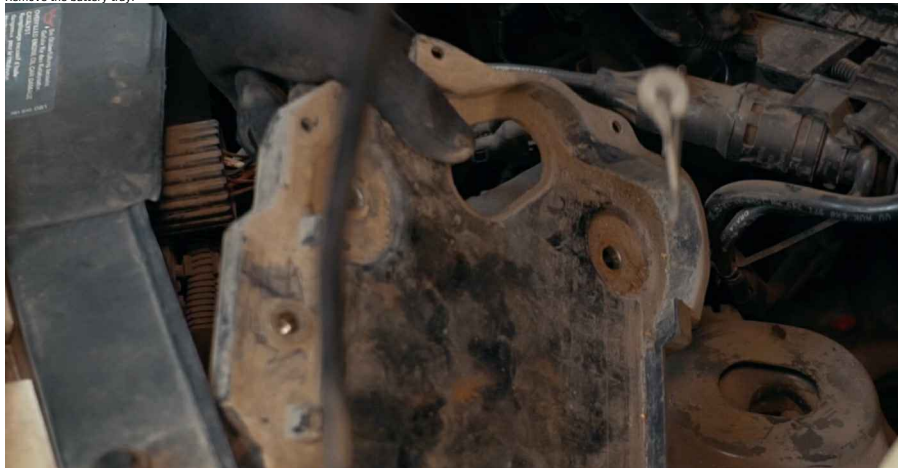
9 Disconnect the clutch cable.
