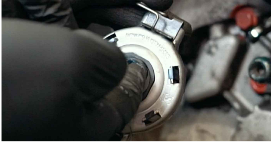
63 Install the new release bearing.
