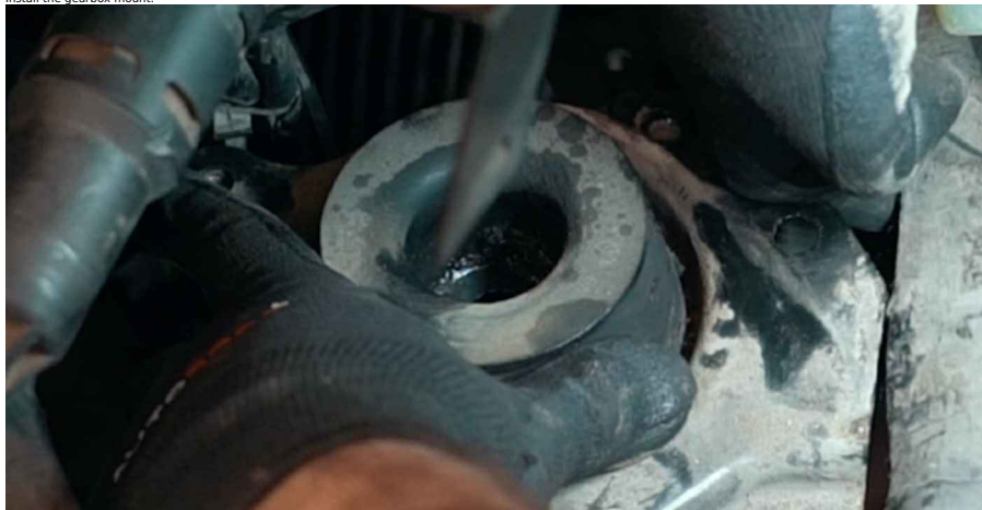
73 Screw in the fasteners that connect the gearbox mount to the car body. Use a drive socket #18. Use a ratchet wrench.
