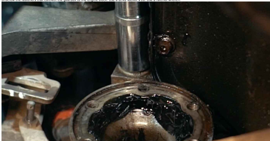
48 Move the gearbox aside.
