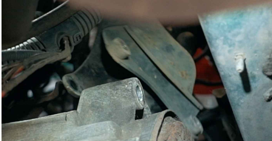
47 Unscrew the fasteners that connect the gearbox to the engine block. Use a drive socket #18. Use a ratchet wrench.
