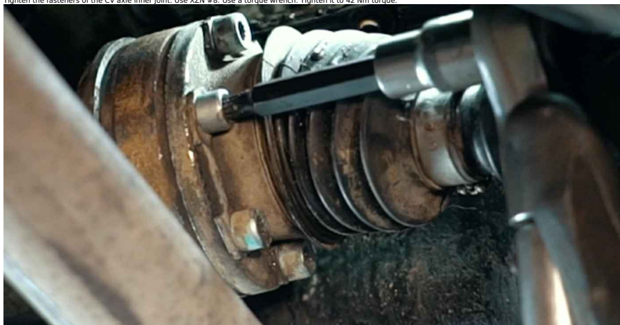
94 Install the fastening nut.
