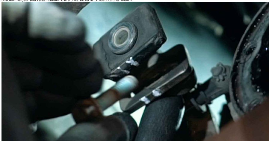
34 Remove the gear shift cable retaining clip. Use a flat screwdriver.
