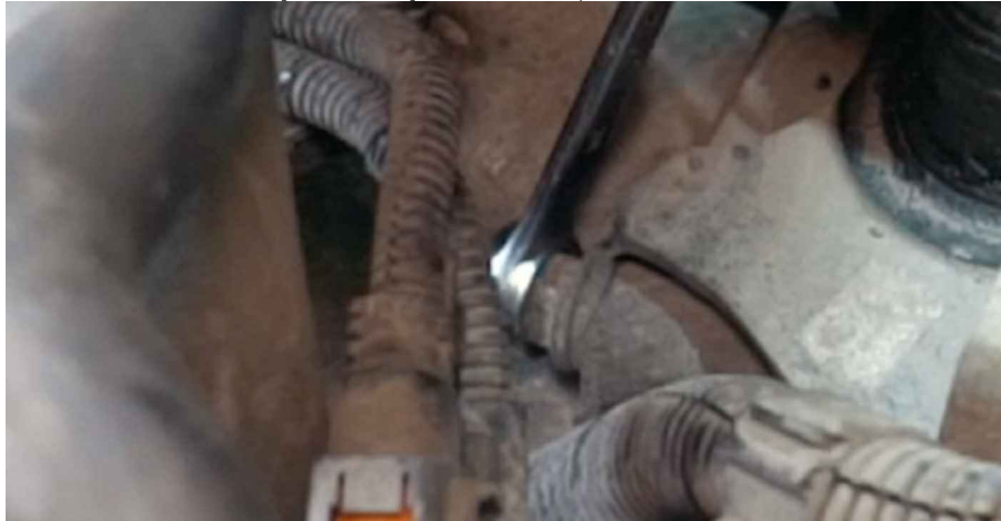
46 Remove the bottom gearbox mount.
