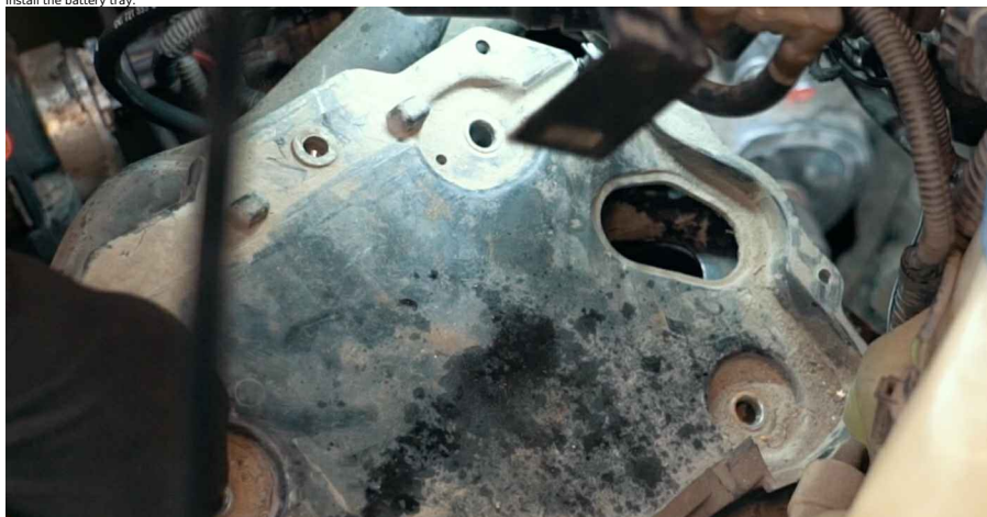
116 Screw in the battery tray fasteners. Use a drive socket #10. Use a ratchet wrench.
