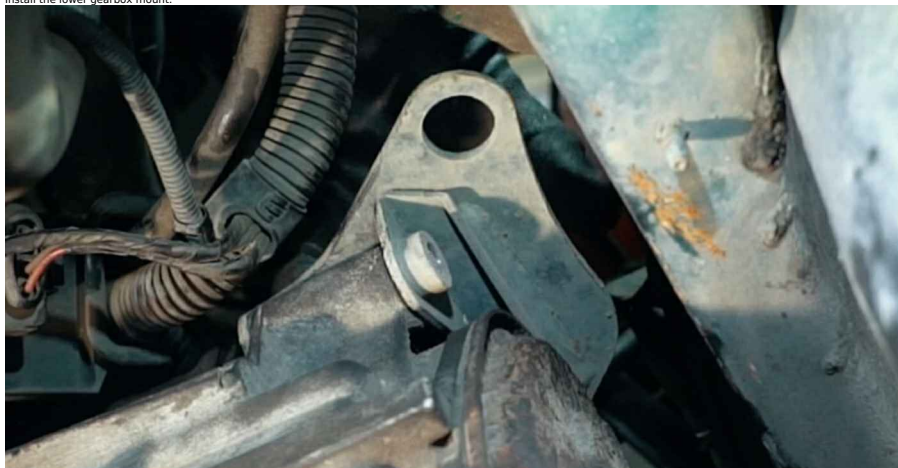
70 Screw in the fasteners that connect the gearbox mount to the gearbox. Use a combination spanner #16.
