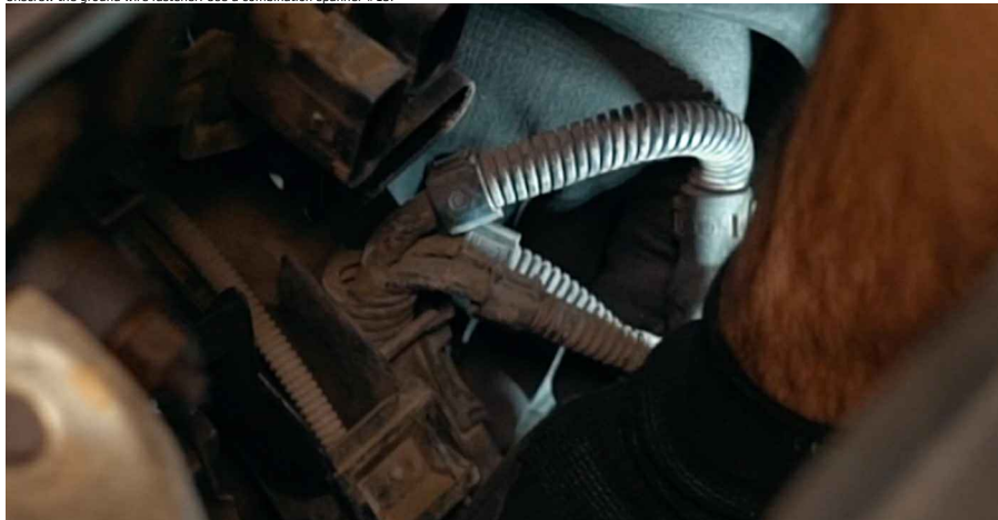
13 Disconnect the ground wire.
