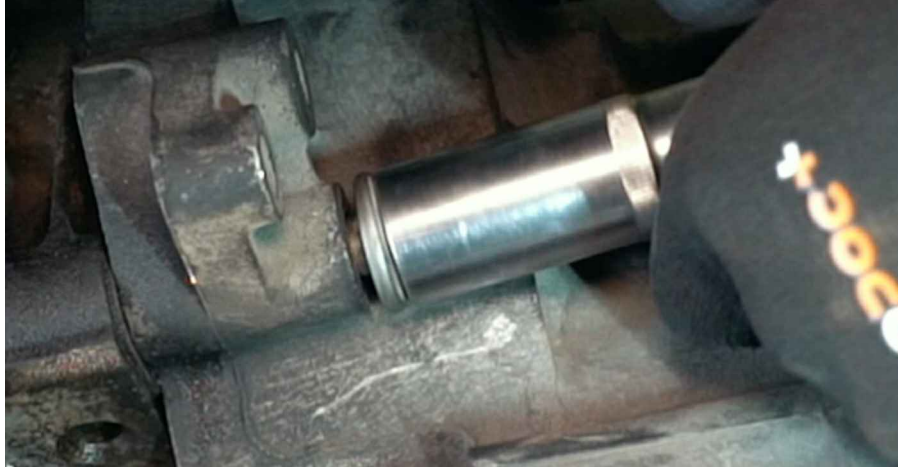
68 Tighten the fasteners that connect the gearbox to the engine block. Use a drive socket #18. Use a torque wrench. Tighten it to 64 Nm torque.
