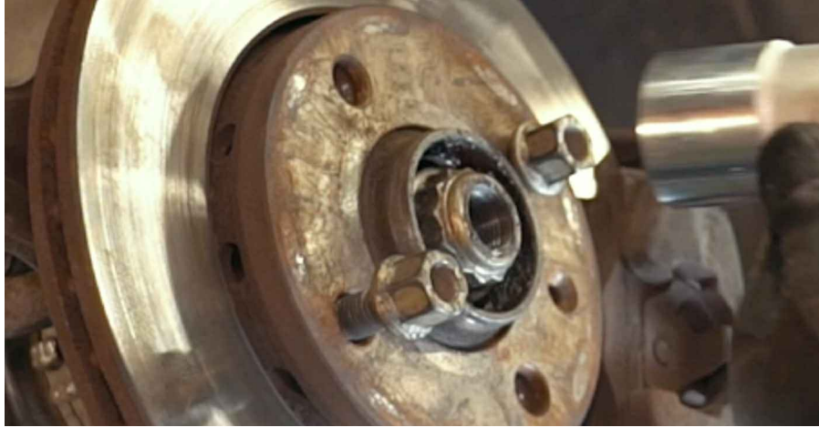
95 Screw in the nut of the CV axle. Use a drive socket #30. Use a ratchet wrench.
