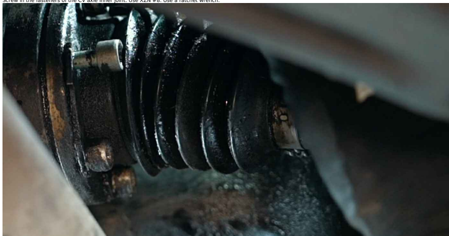
89 Clean the splines of the drive shaft CV joint. Use a wire brush. Use WD-40 spray.
