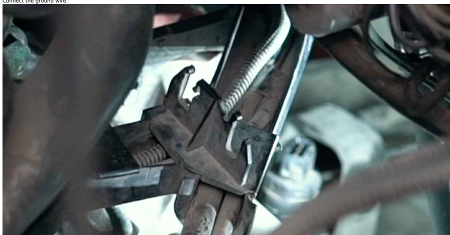
111 Screw on the ground wire fastener. Use a combination spanner #13.
