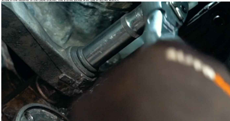
85 Tighten the fastener of the cable bracket. Use a drive socket #16. Use a torque wrench. Tighten it to 22 Nm torque.
