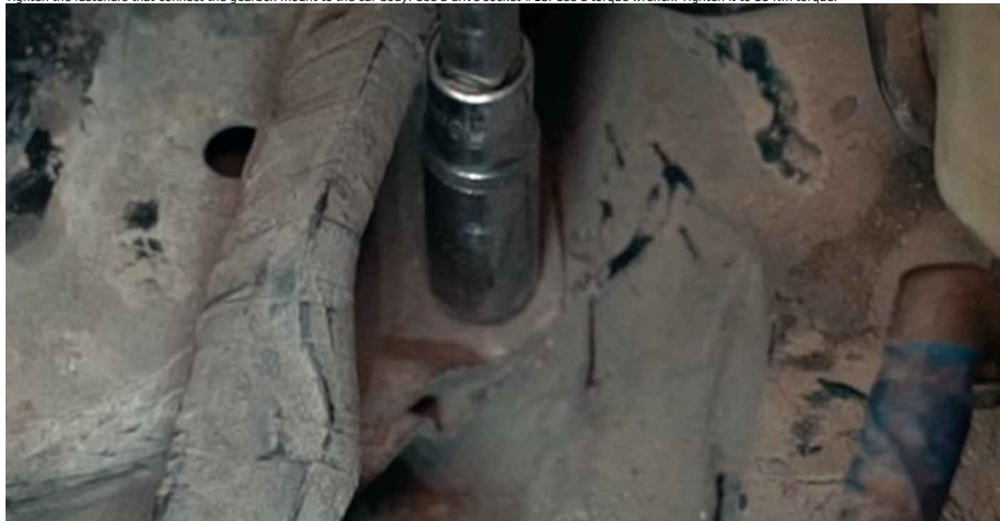
75 Tighten the fasteners that connect the gearbox mount to the gearbox. Use a drive socket #18. Use a torque wrench. Tighten it to 69 Nm torque.
