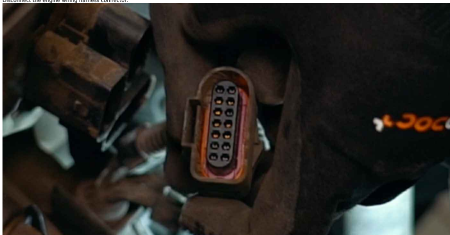
11 Detach the engine wiring harness.
