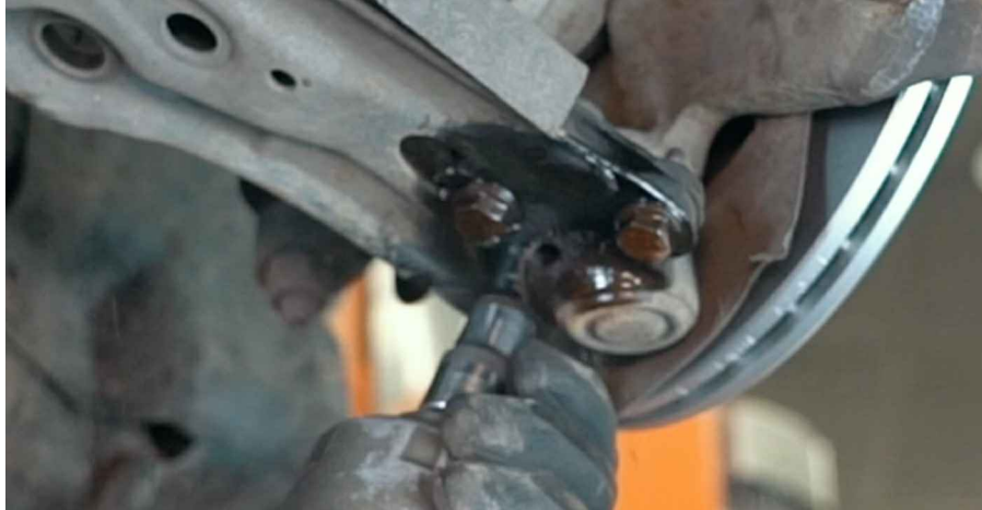
27 Disconnect the ball joint from the control arm.
