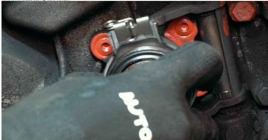
52 Unscrew the pressure plate fasteners. Use 12-point socket No.9. Use a ratchet wrench.
