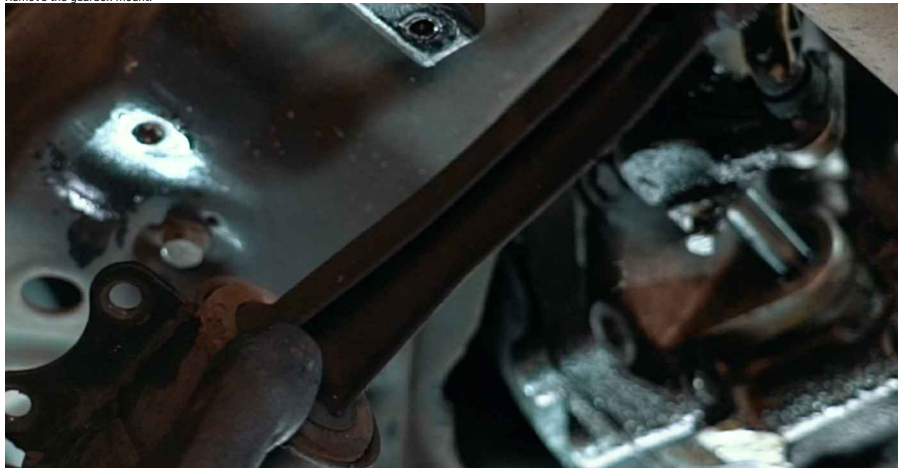
40 Support the gearbox. Use a hydraulic transmission jack.
