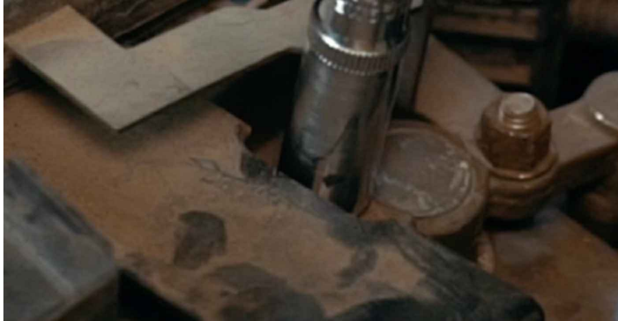
4 Remove the battery terminals.
