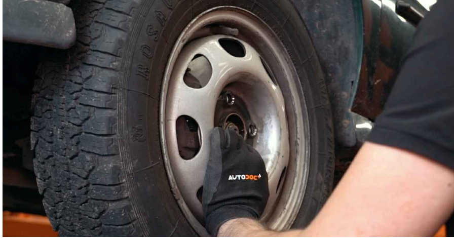
22 Unscrew the fastener connecting the drive shaft to the wheel hub. Use a drive socket #30. Use a ratchet wrench.
