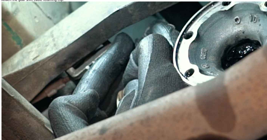
83 Screw in the gear shift cable fastener. Use a drive socket #13. Use a ratchet wrench. club.hatdog.co.uk 21-32
