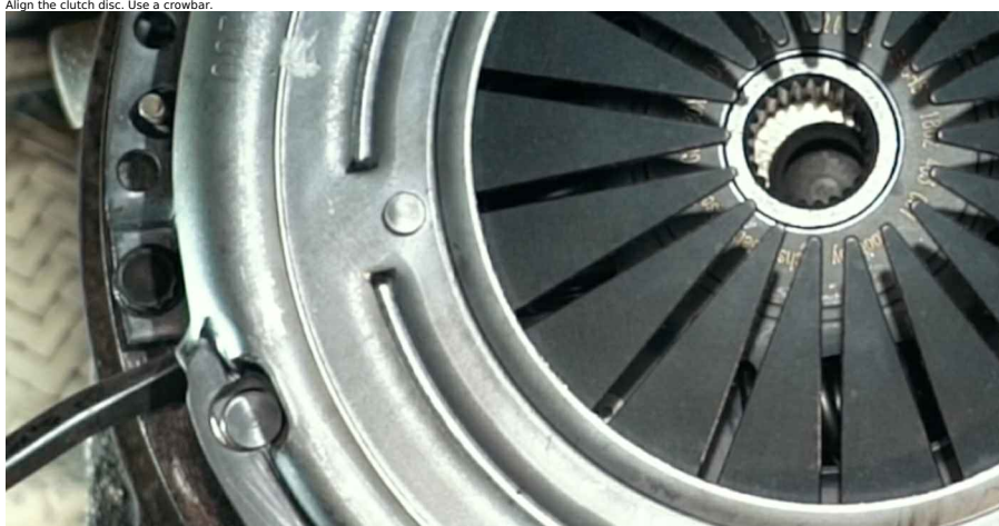
57 Align the clutch disc. Use a crowbar.
