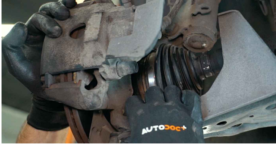
91 Attach the ball joint to the control arm. Use a pin punch.
