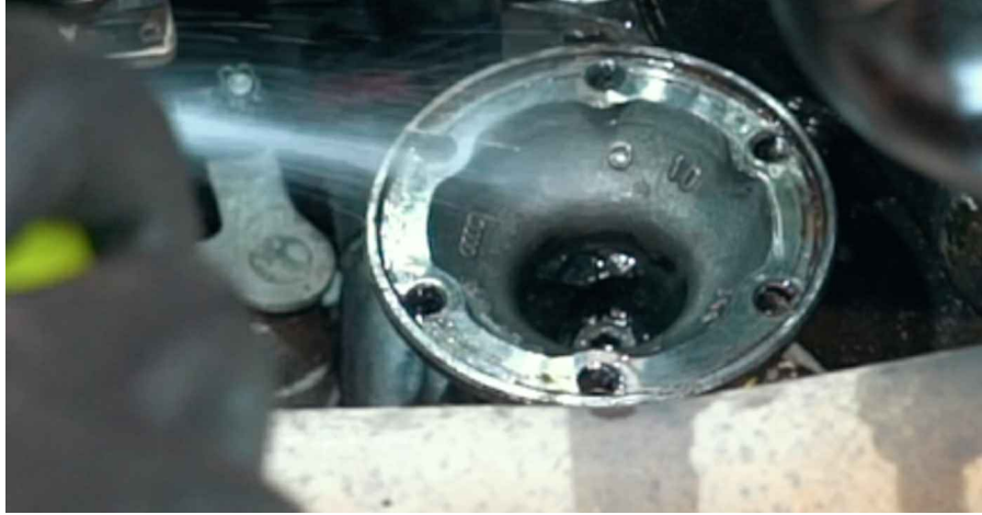
87 Install the drive shaft.
