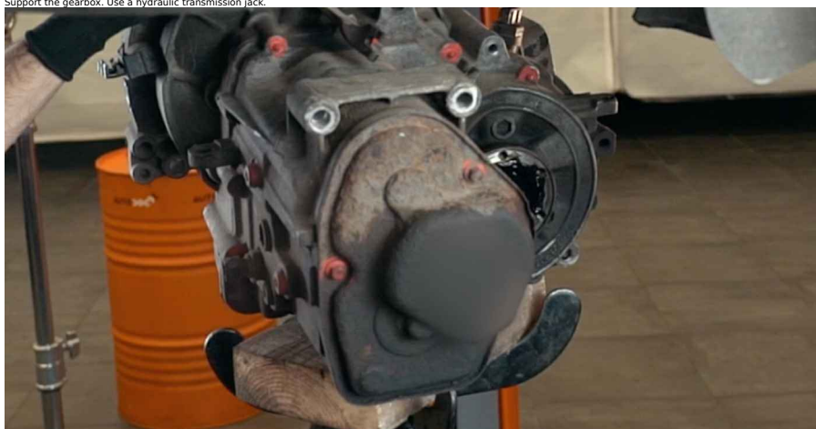
65 Install the gearbox.
