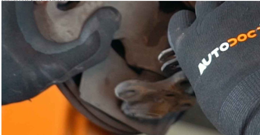
28 Detach the driveshaft from the steering knuckle.
