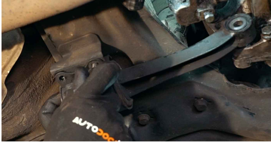
78 Screw in the fasteners that connect the gearbox mount to the subframe. Use a drive socket #13. Use a ratchet wrench.
