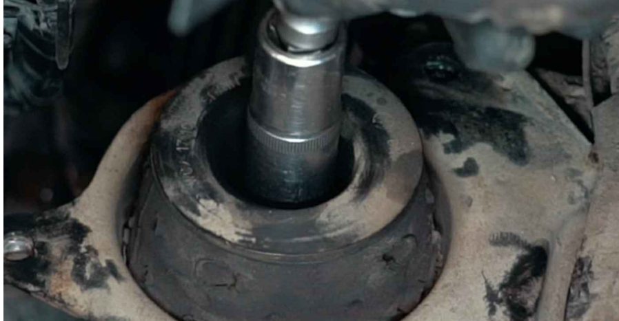
74 Tighten the fasteners that connect the gearbox mount to the car body. Use a drive socket #13. Use a torque wrench. Tighten it to 38 Nm torque.
