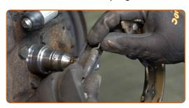
Disconnect the parking brake cable. Use a crowbar.
