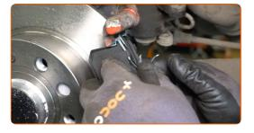
Install the brake caliper and fix it. Use a combination spanner #13. Use a combination spanner #15.
