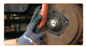
Remove the wheel hub nut cap. Use a crowbar. Use a hammer.
