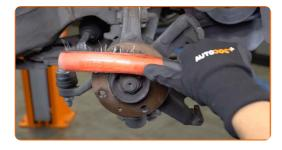
Clean the brake caliper bracket of dirt and dust. Use a wire brush. Use a brake cleaner.
