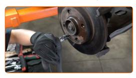
15 Remove the brake disc.
