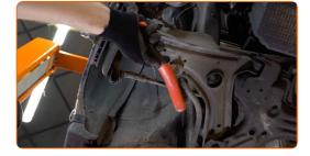
Unscrew the fastener connecting the stabilizer bar with the control arm. Use a drive socket #13. Use a ratchet wrench.
