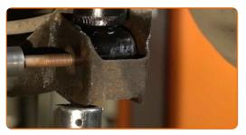
Screw in the lower fastener of the shock absorber. Use a drive socket #16. Use a ratchet wrench.
