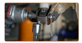
Unscrew the upper fastener of the shock absorber. Use a drive socket #16. Use a ratchet wrench.
