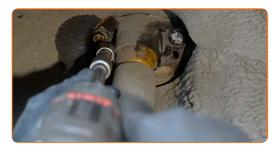
Remove the fastening bolt.
