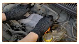
Take out the ignition coil from the spark plug well. Use a crowbar.
