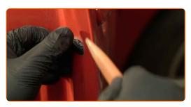
Unscrew the fastener of the exterior door handle. Use Torx T20. Use a ratchet wrench.
