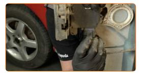
Remove the door lock. Use a flat screwdriver.
