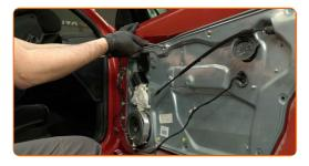
Tighten the door lock fasteners. Use XZN #8. Use a torque wrench. Tighten it to 20 nm torque.
