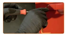
17 Remove the handle-to-lock cable. Use a flat screwdriver.
