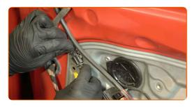
Detach the wiring harness from the protective cover of the door. Use a clip removal tool.
