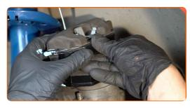
Install the brake caliper and fix it. Use HEX No.H7. Use a torque wrench. Tighten it to 28 Nm torque.
