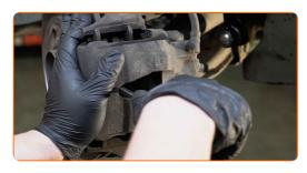
10 Remove the brake caliper.
