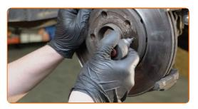
14 Remove the brake disc.
