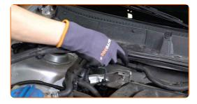
Unscrew the plastic panel fasteners. Use a Phillips screwdriver.
