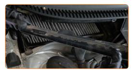
Press on the cabin filter retainer to release it.
