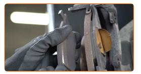
Clean the brake disc fasteners. Use a wire brush. Use WD-40 spray.
