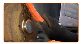
Treat the contacting surface. Use copper grease.
